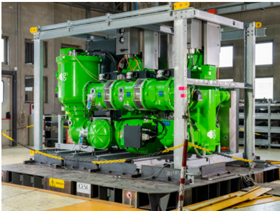
Seismic tests performed on shaking table at CESI Laboratory, in Italy.
