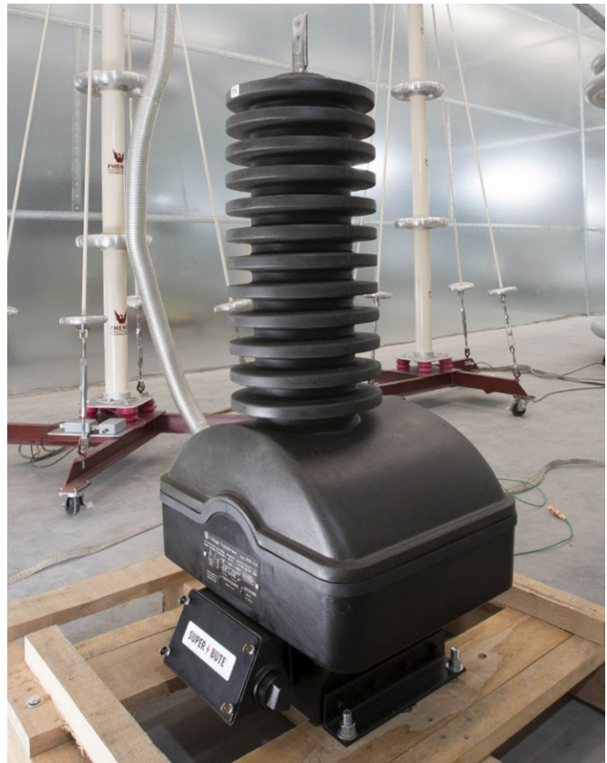
Impulse and partial discharge testing at the Clearwater Test Lab
