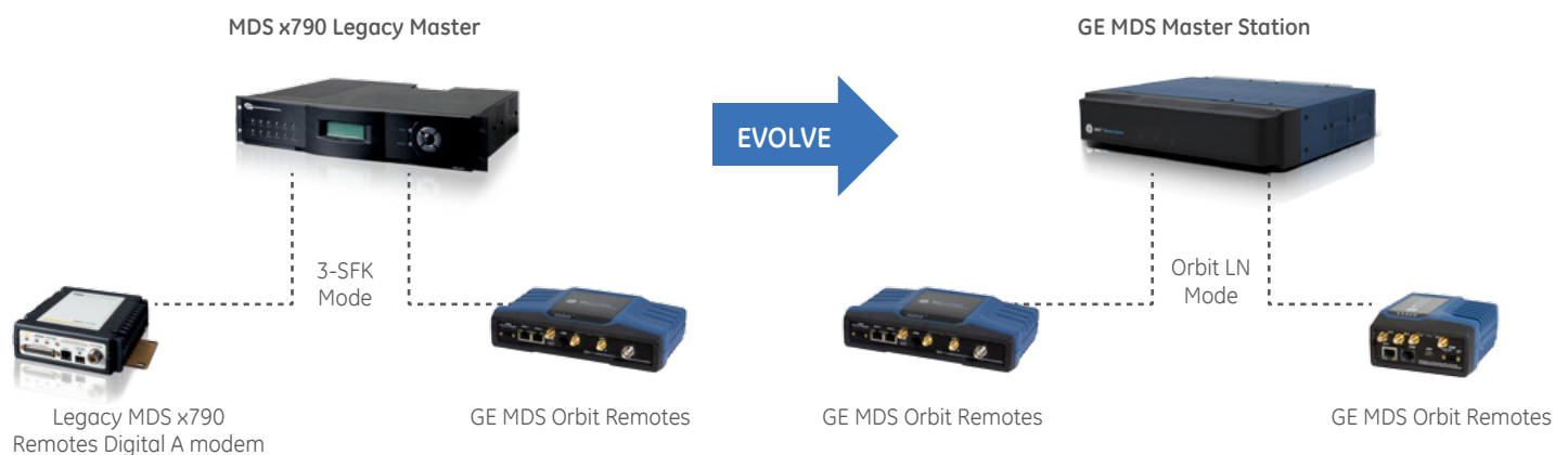
Figure 3: Backwards compatibility firmware in the GE MDS Orbit remote, allowing x710 networks to migrate to the MDS Orbit Platform through the legacy Master Station.
