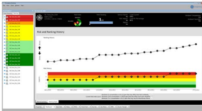
Figure 14: Transformer dashboard as depicted in GE's Perception Fleet Software. showing colour coding and trending of a transformers Risk Index
