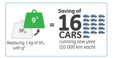
Replacing 1 kg of  $SF_6$  with the corresponding mass of  $g^3$  is the carbon equivalent of removing 16 cars running one year\*\*\*. The potential for global warming reduction is further underscored when you look at the sheer quantity of  $SF_6$  installed worldwide. 10,000 tons of  $SF_6$  are installed each year, with 80% concentrated in the transmission industry.
