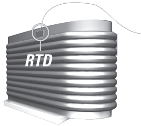
Figure 7. RTD connection for Thermal Protection and Biasing.
