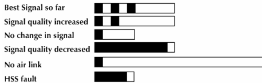
Figure 2-6. Beeper Sequence for ODU Alignment
