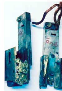
Severely Damaged Brush Holders
