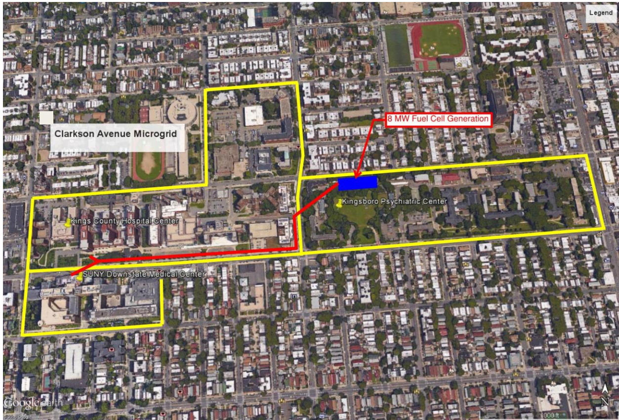
Simplified Layout of Clarkson Avenue Microgrid Showing Facilities and Routing of Electrical Connections Figure 2-1
