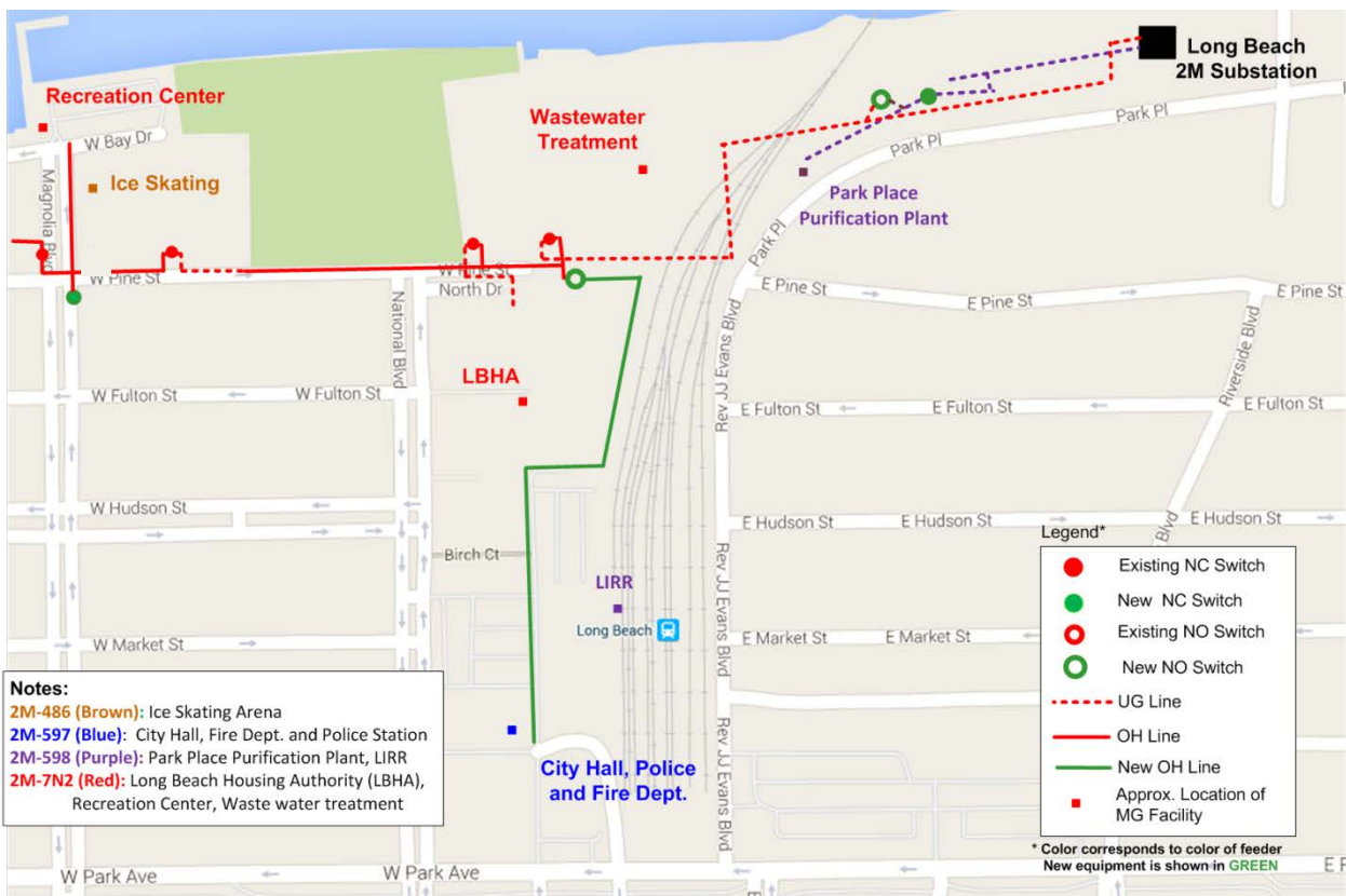
Simplified Layout of Long Beach Microgrid Showing Facilities and Routing of Electrical Connections Figure 2-1
